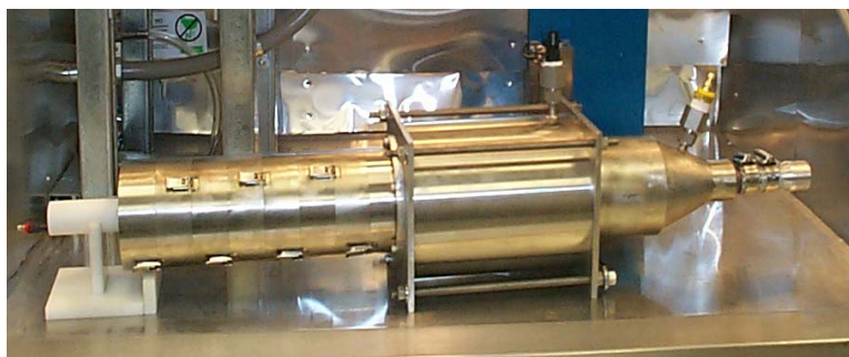
Figure 2. Coaxial tube/wire ESP device developed by InnovaTek for a Swiss company conducting toxicology studies.
